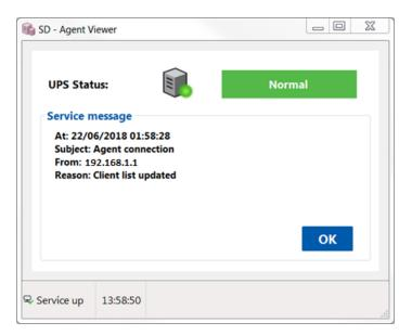
This application indicates the status of the UPS and the SD Agent service. When it is running the status icon is displayed in the systray bar. Double clicking on the icon opens the Viewer window.
