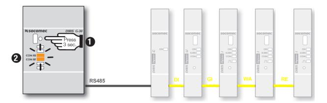
• (3) Wait until the end of the scan, i.e. when the two COM LEDs on the DIRIS G-30 stop flashing:
