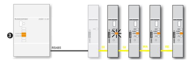
• (4) Automatically address all the slaves whose COM LEDs are not flashing, by pressing and holding down their button for 3 seconds (until their COM LED starts flashing). There is no need to press the button on a slave whose COM LED is flashing, because they already have a unique JBUS/MODBUS address on the bus:
