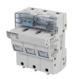
RMS are modular fuse disconnect switches for cylindrical fuses. They provide safety disconnection and protection against overloads and short-circuits in any low voltage electrical circuit.
