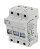
RMs are modular fuse disconnect switches for cylindrical fuses. They ensure safe disconnection and protection against surges and short-circuits in any low voltage electrical circuit.
