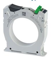
Residual core transformers, including the active conductors, establish the differential sum of the vector currents to detect leakage currents.
