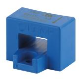
DC current sensors measure the DC load currents of an electrical installation and transmit information to the ldc measurement modules via an RJ12 connection on the side of the module and Molex on the side of the sensor.
