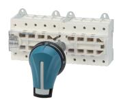
SIRCO VM1 are 3 or 4 pole modular manual transfer switches with visible breaking. They provide on-load transfer between two sources for any low voltage power circuit, as well as safety isolation. Other applications include source inversion (e.g. to change the direction of a motor) or grounding/earthing.
