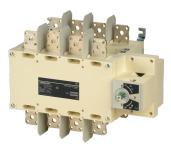
SIRCOVER products are manually operated transfer switches with positive break indication, for open-transition switching (I-0-II) available in 3 or 4 pole. They provide on-load transfer between two sources for any low voltage power circuit, as well as safety isolation by double breaking per pole. Other applications include source inversion (e.g. to change the direction of a motor) or grounding/earthing.
