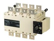
SIRCOVER products are manually operated transfer switches with positive break indication, for open-transition switching (I-0-II) available in 3 or 4 pole. They provide on-load transfer between two sources for any low voltage power circuit, as well as safety isolation by double breaking per pole. Other applications include source inversion (e.g. to change the direction of a motor) or grounding/earthing.
