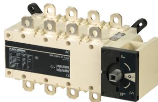
SIRCOVER products are manually operated transfer switches with positive break indication, for open-transition switching (I-0-II) available in 3 or 4 pole. They provide on-load transfer between two sources for any low voltage power circuit, as well as safety isolation by double breaking per pole. Other applications include source inversion (e.g. to change the direction of a motor) or grounding/earthing.
