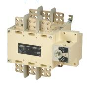
SIRCOVER products are manually operated transfer switches with positive break indication, for open-transition switching (I-0-II) available in 3 or 4 pole. They provide on-load transfer between two sources for any low voltage power circuit, as well as safety isolation by double breaking per pole. Other applications include source inversion (e.g. to change the direction of a motor) or grounding/earthing.
