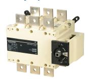
SIRCOVER products are manually operated transfer switches with positive break indication, for open-transition switching (I-0-II) available in 3 or 4 pole. They provide on-load transfer between two sources for any low voltage power circuit, as well as safety isolation by double breaking per pole. Other applications include source inversion (e.g. to change the direction of a motor) or grounding/earthing.
