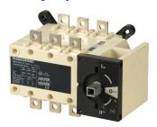
SIRCOVER products are manually operated transfer switches with positive break indication, for open-transition switching (I-0-II) available in 3 or 4 pole. They provide on-load transfer between two sources for any low voltage power circuit, as well as safety isolation by double breaking per pole. Other applications include source inversion (e.g. to change the direction of a motor) or grounding/earthing.
