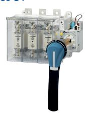
FUSOMAT fuse-combination switches are manually operated 3 or 4-pole load break switches with visible breaking and a remote tripping function.
