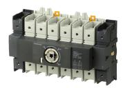
SIRCO M are manually operated 3 or 4 pole modular transfer switches with positive break indication. They provide on-load transfer between two sources for any low voltage power circuit, as well as safety isolation. Other applications include source inversion (e.g. to change the direction of a motor) or grounding/earthing.
