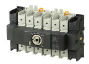
SIRCO M are manually operated 3 or 4 pole modular transfer switches with positive break indication. They provide on-load transfer between two sources for any low voltage power circuit, as well as safety isolation. Other applications include source inversion (e.g. to change the direction of a motor) or grounding/earthing.
