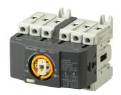
SIRCO M are manually operated 3 or 4 pole modular transfer switches with positive break indication. They provide on-load transfer between two sources for any low voltage power circuit, as well as safety isolation. Other applications include source inversion (e.g. to change the direction of a motor) or grounding/earthing.
