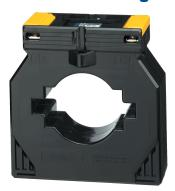
Current transformers deliver to the secondary a standard current proportional to the primary current and adapted to the rating of the associated device. They are equipped as standard with removable terminal covers and double terminals allowing the secondary to be short-circuited without any risk.
