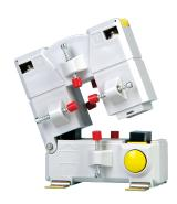
Current transformers deliver to the secondary a standard current proportional to the primary current and adapted to the rating of the associated device. They are equipped as standard with removable terminal covers and double terminals allowing the secondary to be short-circuited without any risk.
