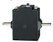
Current transformers deliver to the secondary a standard current proportional to the primary current and adapted to the rating of the associated device. They are equipped as standard with removable terminal covers and double terminals allowing the secondary to be short-circuited without any risk.
